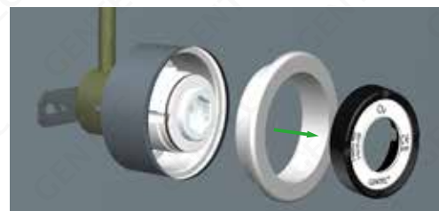
1A. Pull the pressure lid and the decor off
